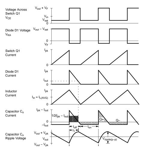
Figure 10. Step–Up Switching Regulator Waveforms
