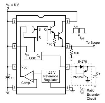
Figure 19. Output Switch On–Off Time Test Circuit
