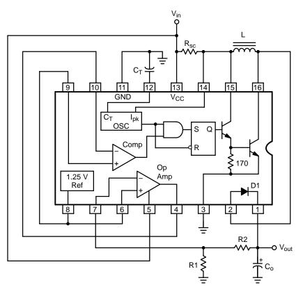
Figure 12. µA78S40 Ripple Reduction Technique
