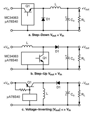
Figure 7. Basic Switching Regulator Configurations
