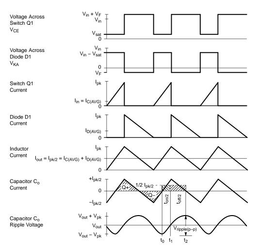
Figure 8. Step–Down Switching Regulator Waveforms
